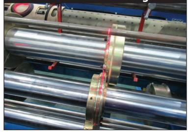
Unique to the Scorpion, it features a laser-assist feature to assist alignment of the slots and scores. Simply set the laser to the correct dimension and then align the scores and slots to the laser.
