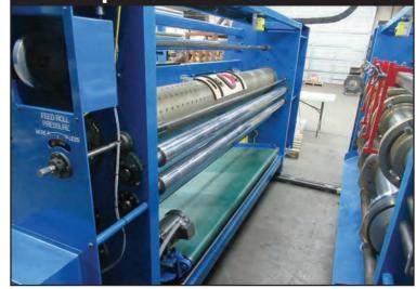
The Scorpion can also be equipped with an optional Rotary Die Cut Station. It features a full two inches of oscillation on the anvil cylinder and oversized eccentrics for stability and long bearing life.
