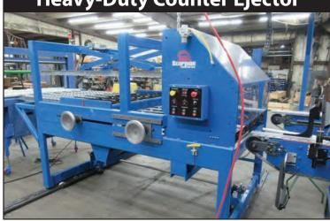
The under-stacking Counter Ejector features motorized hold down adjustment and variable speed for the stacking belts and the outfeed carriage belts, as well as manual side-shift.
