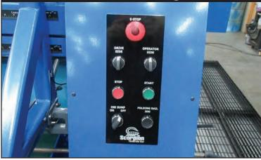
The Scorpion FFG features motorized folding rails adjust including a folding rail jog button.
